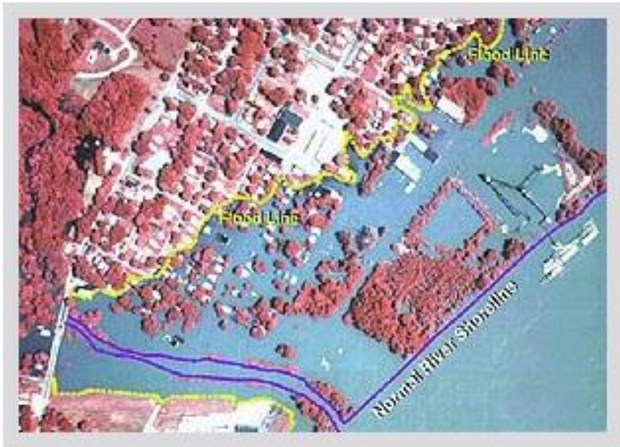
Flood Boundary Extraction
